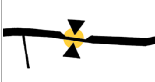
Traffic calming diagram: road narrowing
