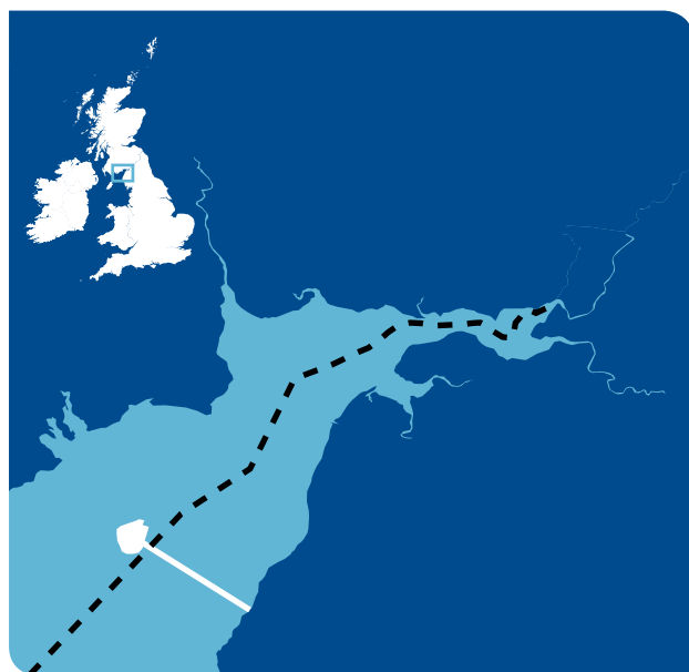
ROBIN RIGG SAND FLAT, AND CABLE ROUTE. THE SEABED CONSISTS OF MOBILE SAND OVER CLAY.
