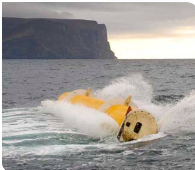
OYSTER HYDRO-ELECTRIC WAVE ENERGY CONVERTER © AQUAMARINE POWER
